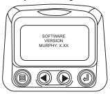
Touch "Menu" to return to "Utilities". Highlight Fault Conversion" using the "Arrows". Touch "Select" to enter the Fault conversion menu.
